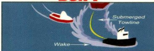
Never pass closely behind a tugboat. Under no circumstances should you ever pass between a tug and its tow! The tow line may be submerged and hard to see.
