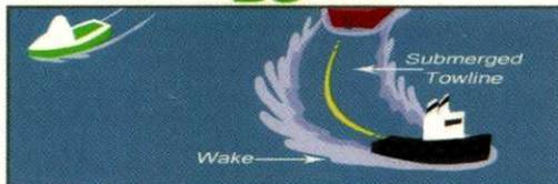
Stay a safe distance from tug boats and keep an eye out for barges in tow. Tug boats can create severe wake turbulence hundreds of yards behind the vessel.
